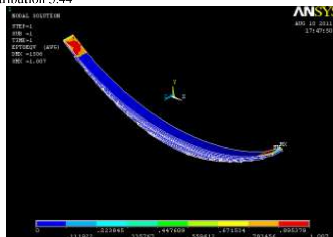
Figure: 8.7 Strain distribution for graphite epoxy composite leaf spring load 6000N
