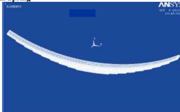
Figure: 7. 1 Mesh model of composite leaf spring
